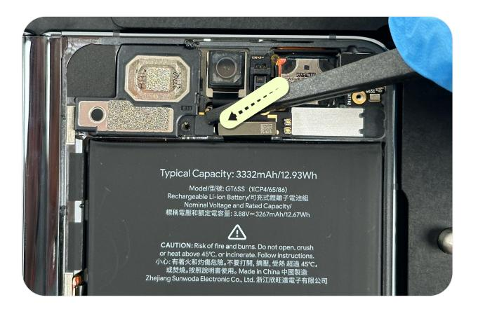
Outer Display Lower Board Flip Cowling with Vibrator
