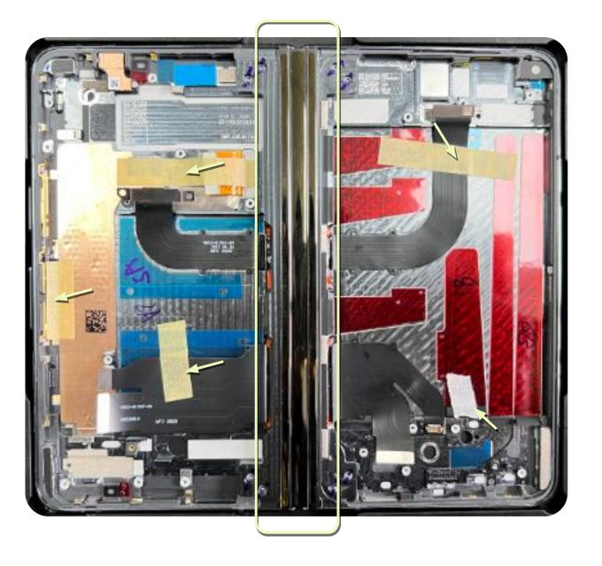
Inner Display Sub Flip cowling with vibrator Flip Battery Lower Board Outer Display Receiver Detune Board Outer Front Camera Upper Board Top Speaker
