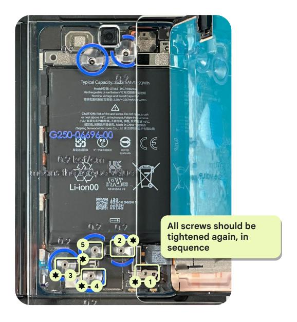
Inner Display Sub Receiver Detune Board Out
