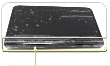
Replace if the protective film is broken. Tear off the PF with device folded.
