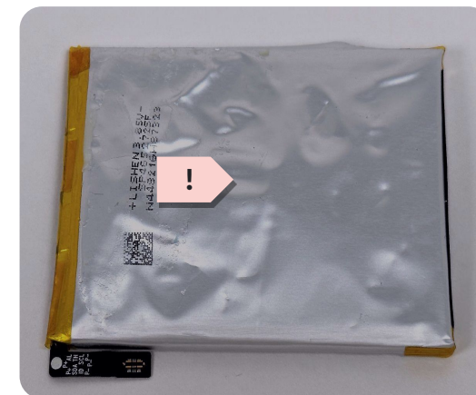
Swelling or electrolyte leakage
