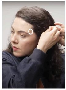
4. Point the camera bar (located below the camera flash) on the smartphone over the center of your forehead. The smartphone will vibrate when in range.
