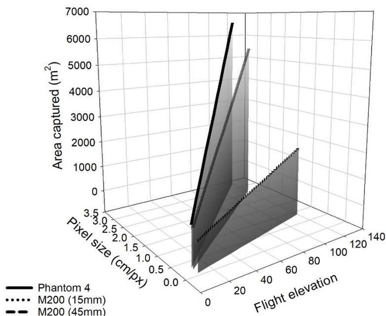
Figure 8: Visualisation of the influence of flight elevation on pixel size at the ground and area captured for three imaging systems with different camera focal lengths.
