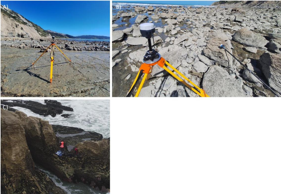
*Figure 5: A) A base station set up on a levelled surveying tripod, B) base station and rover on 2m survey staff and C) personnel taking the GPS coordinates of the GCP.*
