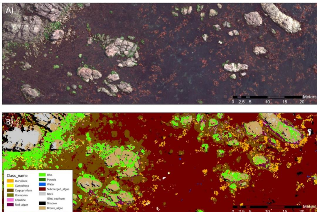
Figure 8: An example of A) multispectral imagery of a rocky shore, and B) the classification of multispectral imagery.
