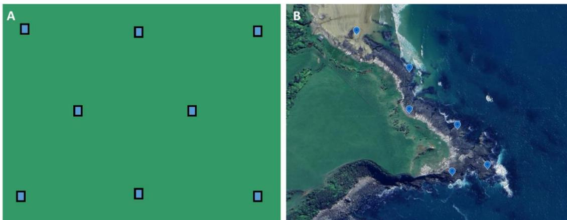
Figure 7: A) An example of ideal GCP configuration across a survey area and B) example of possible GCP locations on a small, narrow rocky reef.
