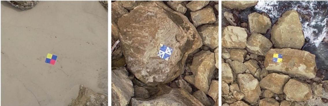
Figure 6: Examples of Ground Control Point (GCP) targets used during aerial drone mapping.
