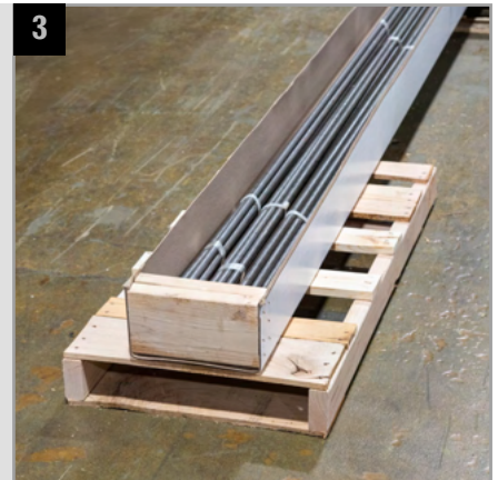
Box (laminated paperboard) is stapled to pallets for secure transit. Wood header blocks are placed on either end of the box to re-enforce the structure of the packaging.
