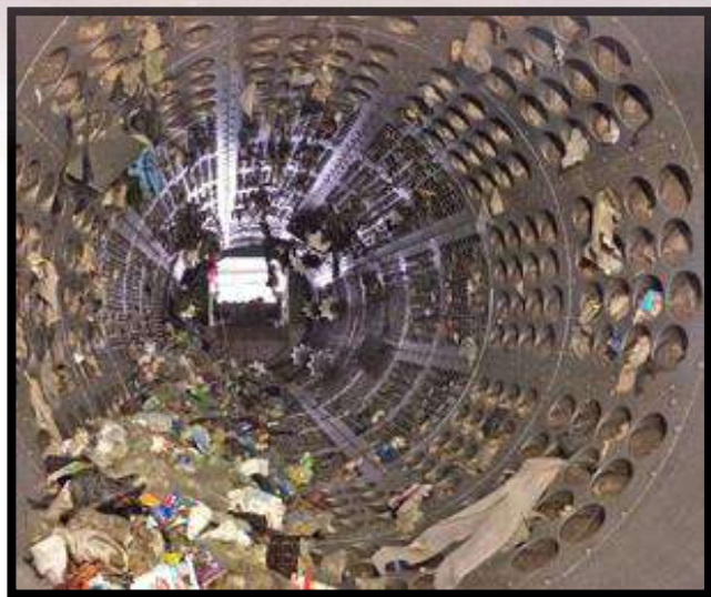
Trommel screen (front and inside view)
