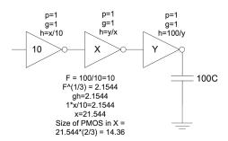
6. Find the optimal normalized delay of circuit.
