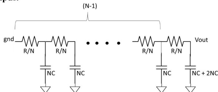
$$\text{tpdf} = \frac{R}{N} X NC + \frac{2R}{N} X NC + \dots + \frac{(N-1)R}{N} X NC + R X 3NC = RC(N^2+5N)/2$$
