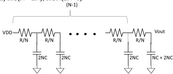
$$\text{tpdr} = \frac{R}{N} \times 2NC + \frac{2R}{N} \times 2NC + \dots + \frac{(N-1)R}{N} \times 2NC + R \times 3NC = \text{RC}(N^2+2N)$$
