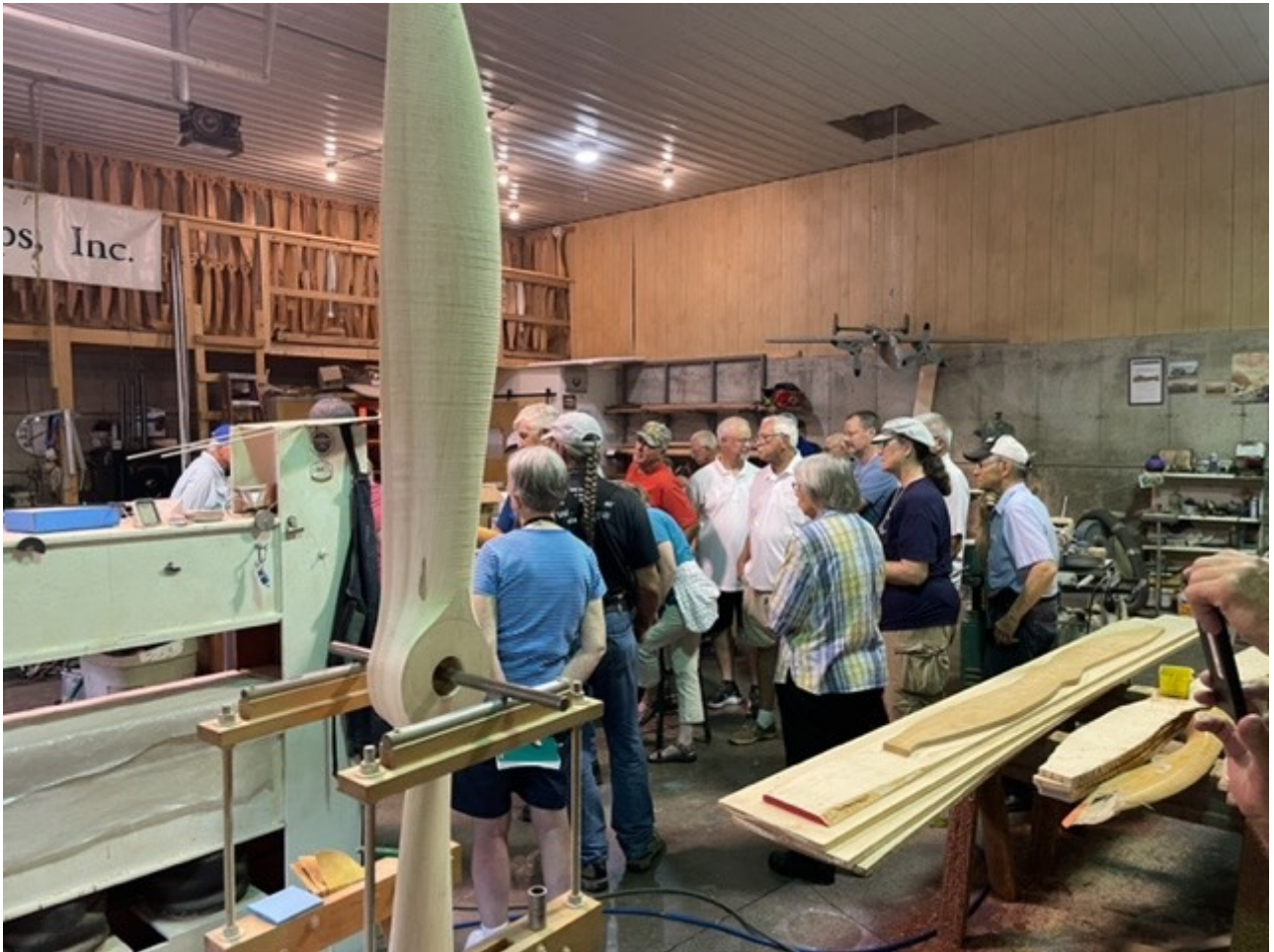
Here's most of our group listening to Alaina. You can get an idea of the size of the shop/factory from the picture. In the foreground is her propeller balancing station. She balances a prop to less than the weight of a Post-It note stuck near the propeller hub.
