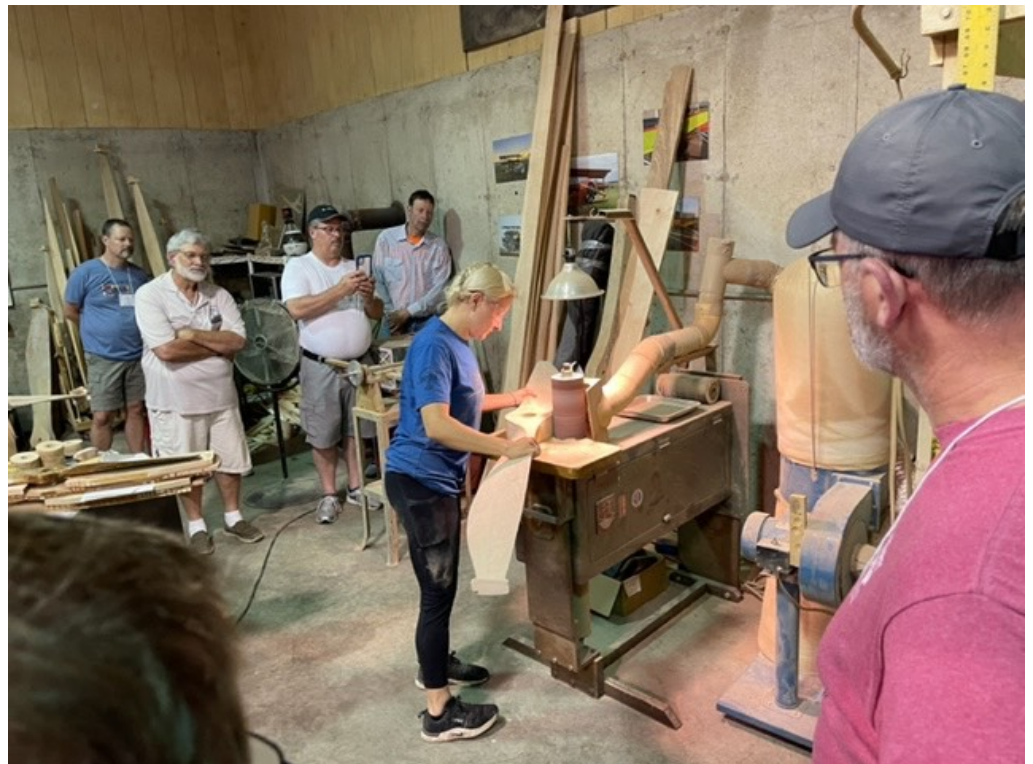
Alaina sanding a propeller. It's lying on the sanding table, but much of the sanding is done by lifting and holding the propeller while sanding it freehand. Alaina isn't a large lady, but she gets a workout and must be plenty strong.
