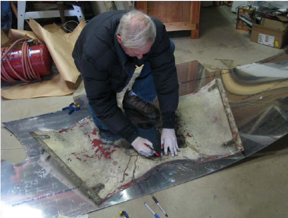
Look how grubby the old part was...worthy of the Utilitarian (Ugly) Award I received for Headwinds years ago. Makes a good pattern, though.
