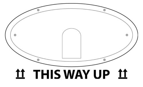
B: Mark your wall with the hole positions to match the mounting plate, as shown in the diagram below.
