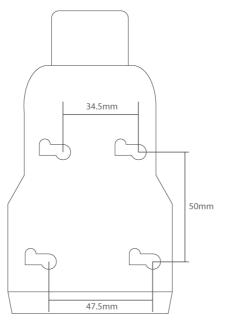
C: Using an 8mm drill, create the 4 mounting holes as marked in the previous step. The holes should be approximately 3.5cm deep.
