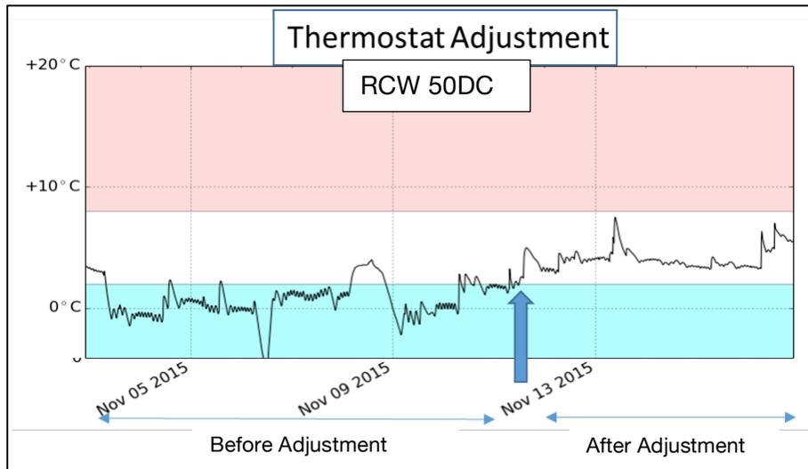
**Figure A:** Screenshot of ColdTrace dashboard showing temperature data from a Dometic RCW 50DC model fridge experiencing cold and freezing excursions before the thermostat adjustment, then performing in range after the adjustment.
