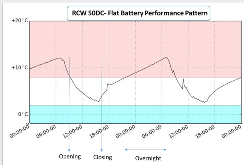
**Figure F:** Screenshot of ColdTrace dashboard showing 48 hours of temperature data from a **solar fridge with flat battery**. At opening and closing time, when facility personnel check the temperature of the fridge, the temperature appears between 2-8° C. However, temperature excursions occur overnight.
