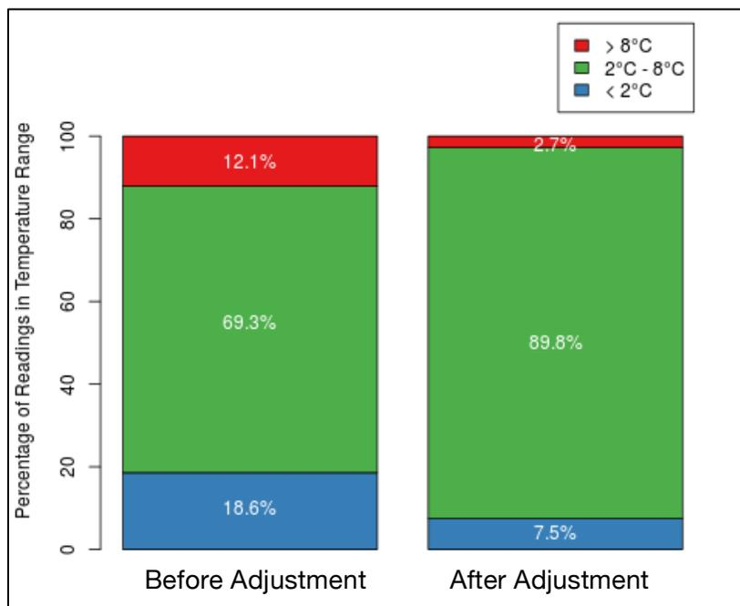
**Figure C:** After remote diagnosis and fix of thermostat adjustment, **fridge uptime at the 8 facilities was increased by 30%**. Heat exposure was reduced by 78%, and cold exposure was reduced by 60%. (n = 8 facilities)
