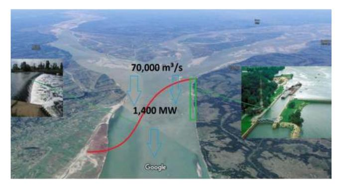
Cascading hydroelectric power plant at this site has an installed capacity of 1,400 MW with a fast-lock for the vessels passage
