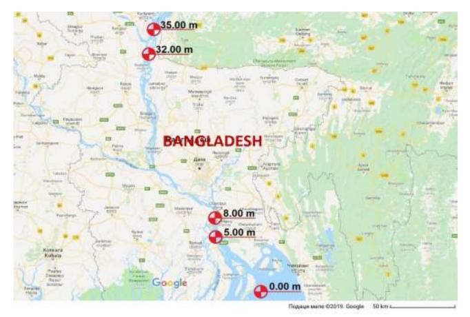
The wetland area will be given to the nature until a height of up to 5m above the sea level, a position where the first cascading hydropower plant is built that creates a water slowdown of 3m, marked at 8m above the sea level
