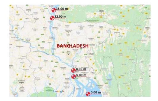
The wetland area will be given to the nature until a height of up to 5m above the sea level, a position where the first cascading hydropower plant is built that creates a water slowdown of 3m, marked at 8m above the sea level
