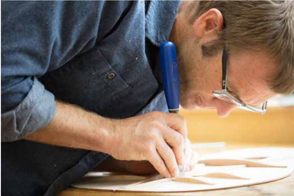
Master Guitar Designer Andy Powers with guitar top featuring V-Class bracing
