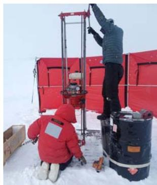
Figure 3. Left, 8m rock core recovered from beneath 150 m of ice at Pirrit Hills in 2016-17 using the ASIG drill (J. Stone photo). Right, Winkie drill at Ohio Range in 2016-17 (IDDO photo).
