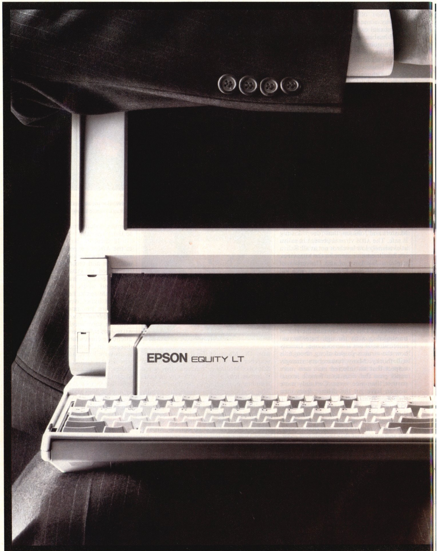
Epson Equity LT. 640K RAM, NEC V30 microprocessor, 4.77/10MHz clock speed, two expansion slots, numeric keypad, CGA and serial/parallel ports, 12.2 lbs., one year limited warranty, optional internal modem. Epson is a registered trademark of Seiko Epson Corporation. Lap-Link is a trademark of Traveling Software, Inc. MS is a registered trademark of Microsoft Corporation. Equity is a trademark of Epson America, Inc., 2780 Lomita Blvd., Torrance, CA 90505. (800) 421-5426.
