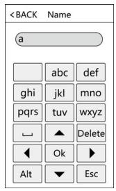
Touch 'Alt' to switch capital/small letter or number, after finished, touch 'Ok' to save it **How to input punctuation:** when the input method is in capital/small letter state, touch '—' to select what you want to input. The first one is space, the second is dot and so on
