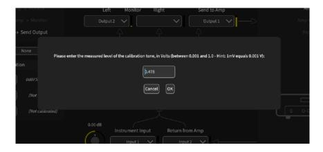
Next, you should calibrate the Instrument Input. While the accuracy of the capture is not affected by this step, following it ensures that when in setup or audition mode your guitar signal reaches the real amp or pedal with no additional gain or attenuation coming from your audio interface. This makes tweaking (prior to running the capture) and evaluation (when auditioning) easier, since the signal reaching your amp or pedal will be the same as if you plugged in directly.
