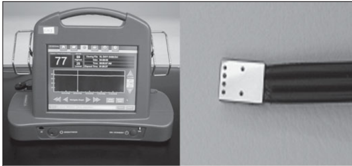
Figure 1. The ViOptix tissue oximeter data is displayed on a windows based console with a touch-screen, user friendly interface (left). The probe (right) emits two wavelengths of light and measures reflected light.
