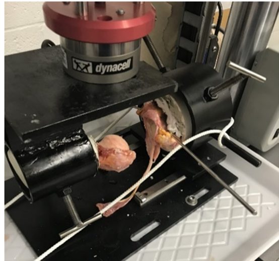
Fig 1. Testing apparatus. The humerus is mounted to the Instron Electroplus 1000, which provides a force to translate the humeral head over the glenoid. The glenoid is mounted to a low-friction sliding platform with a pulley system providing 22.5 N of joint compression force.
