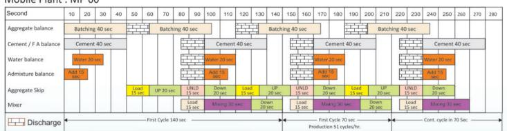
NOTE: Production Capacity based on 1 m³ cycles of standard concrete with 4 aggregates (Max. 2000 kg/m³), 1 Cement (Max. 300 kg/m³), 1 water (Max. 160 kg/m³) & 1 admixture (Max. 4 kg/m³), 30 sec mixing time, 20 sec discharge time normal slump 70 - 130 mm.
