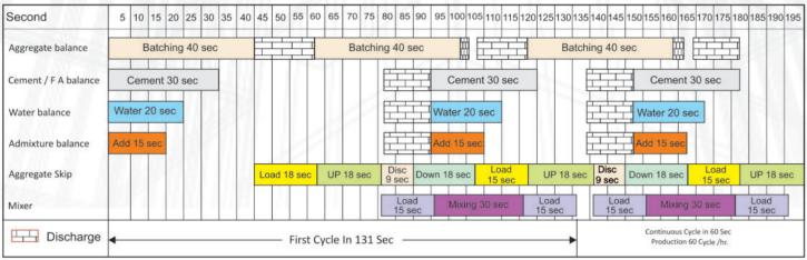
NOTE: Production capacity based on 0.5 m³ cycles of standard concrete with 4 aggregates, 1 cement, 1 water, 1 admixture; slump 70 - 130 mm.
