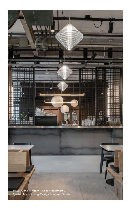
PRESS is made of fat, chunky coils of pure and clear glass, pressed in iron moulds under tons of pressure to create heavyweight grooved glass artefacts. Bold in silhouette and simple in function, the ribbed glass of PRESS lights refracts and diffuses the interior light source from the integrated LED and projects linear and stripy patterns across its surroundings
