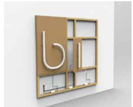
3. Fix panel b and connect panel i to power source.
