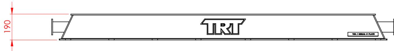
TRT Crane Pads evenly distribute outrigger crane loads. Quality engineering ensures all TRT Crane Pads adhere to the CICA industry standards.
