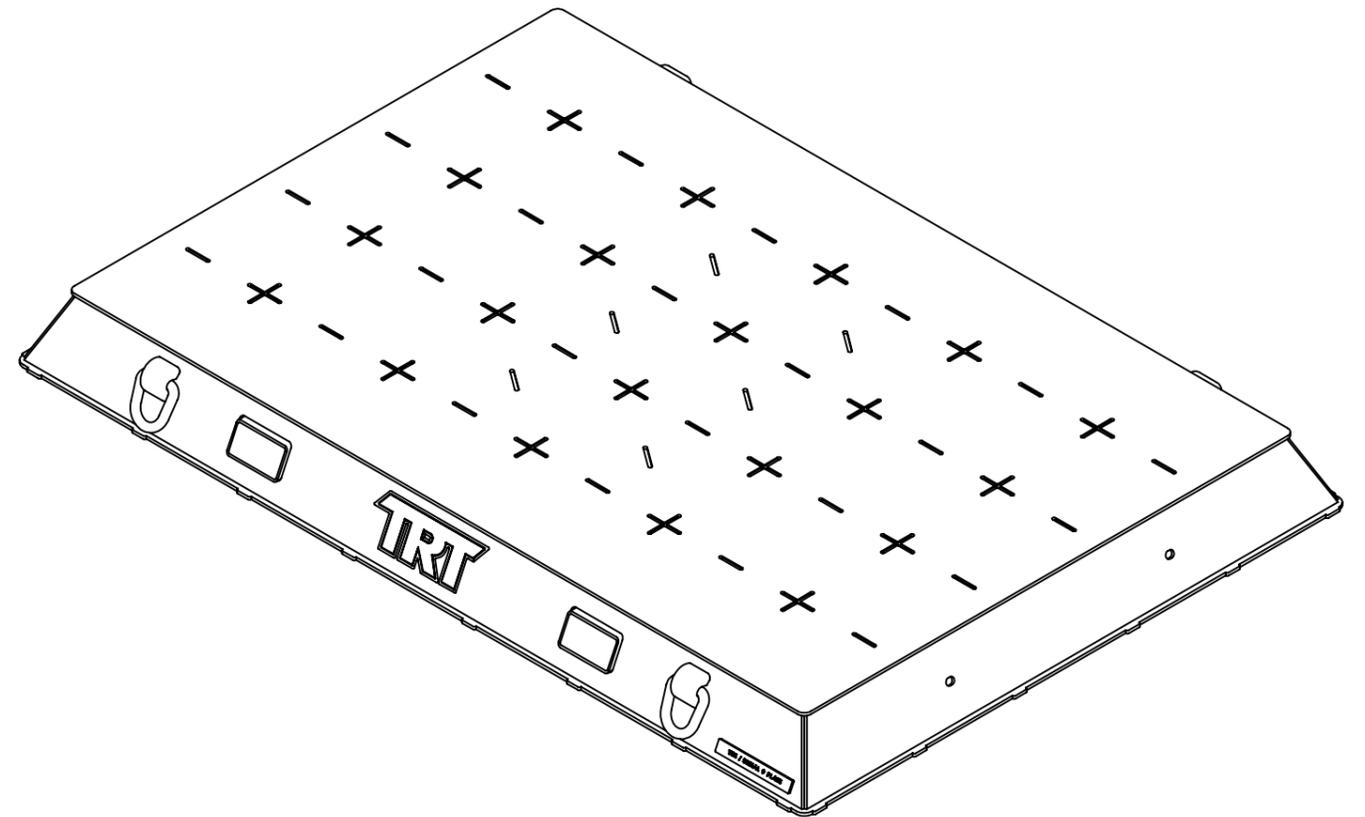
TRT Crane Pads evenly distribute outrigger crane loads. Quality engineering ensures all TRT Crane Pads adhere to the CICA industry standards.
