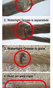
1. Crack on Watertight Grease
