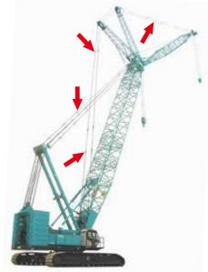
Watertight Grease: The Watertight Grease is being applied on guy cable clamped section at manufacturing. But oils/fats ingredient in the Watertight Grease would be reduced by age or dust. And the Watertight Grease gets hard like caulking.
