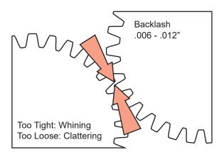
Backlash is necessary to allow gears to mesh adequately and without undue stress between the gears.
