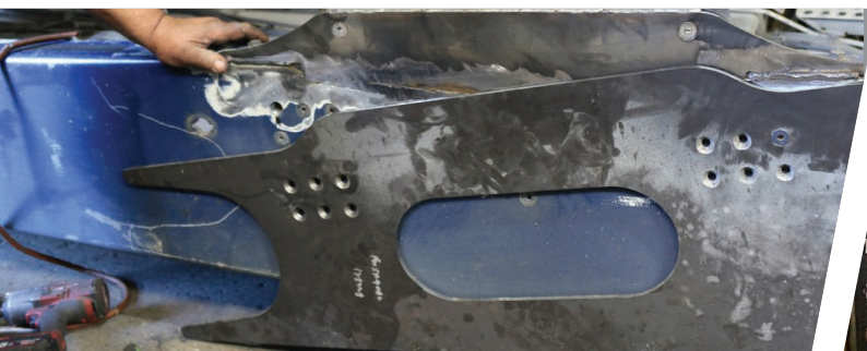
Nice bit of work by the TRT Repair Bay. This trailer unit was in 2 parts until George and Steve worked their welding magic. The next step was adding a custom-made piece for more support.
