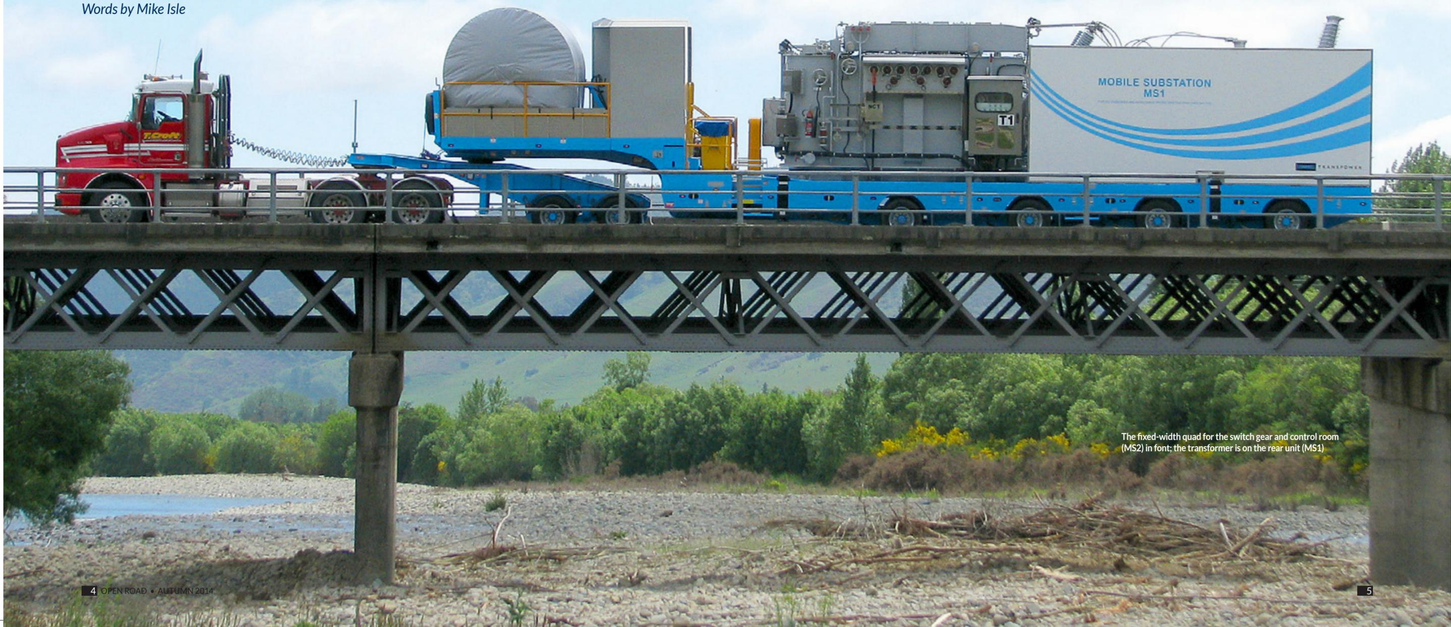
The fixed-width quad for the switch gear and control room (MS2) in front; the transformer is on the rear unit (MS1)
