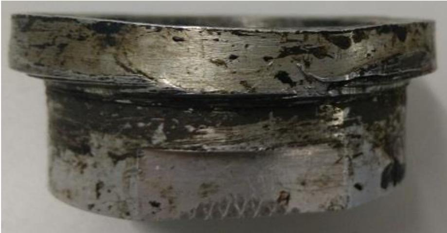
*Figure 2: The damage in the old die adapter plate*
