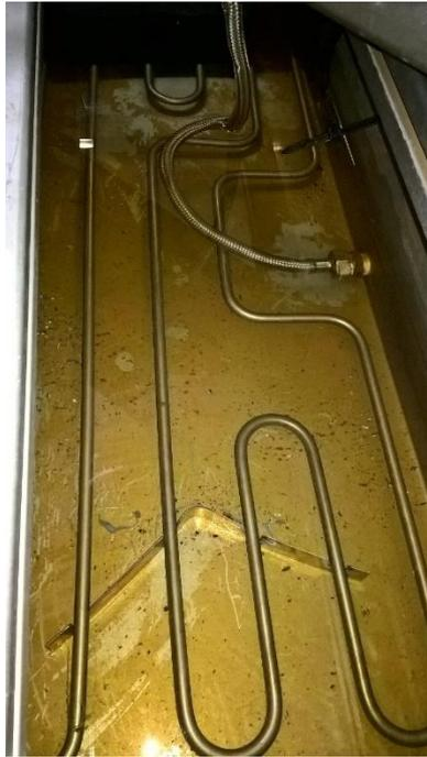
*Figure 5: The new heating element in the cooling bath, resting on supports on the bottom of the bath*
