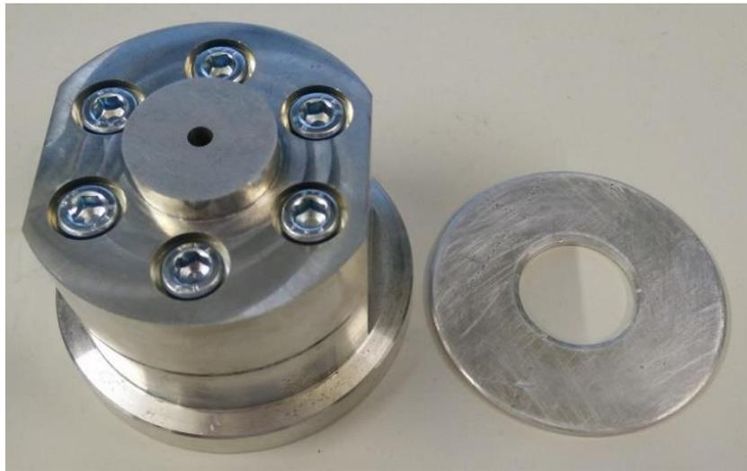
*Figure 3: The aluminium prototype. An additional disc was designed to cover the bolts from getting contaminated with molten plastic while in use to ensure easy dis-assembly.*
