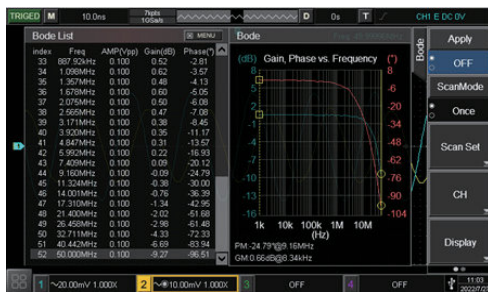
Bode plot option available for loop analysis
