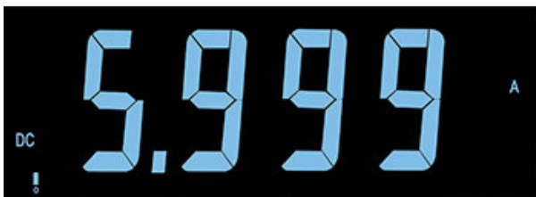
Reading resolution 3½ digits. Maximum count 5,999
