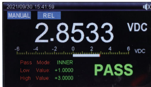
Batch test function. This will help you check components quickly and pass or fail them based on your criteria
