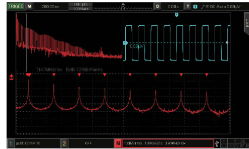
64kpts enhanced FFT for easy frequency domain analysis of signals
