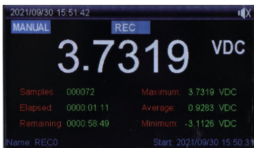
UT8804E digital multimeter has a recording function. Historical data records can be presented in statistics and trend charts.
