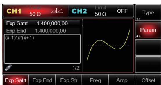
Built-in 16 types harmonic generators
