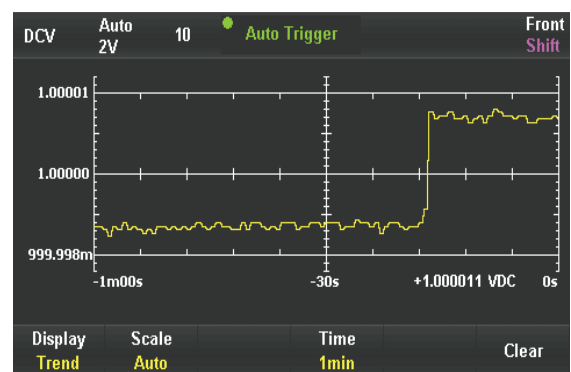
UT8806E supports multiple display modes. Users can observe measurement data through numbers, bar graphs, trend graphs and histograms.
