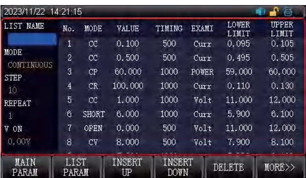
Freely edit test items in List mode to help you implement automated measurement
