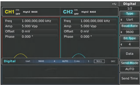
Optional digital signal output interface: SPI, IIC, UART
