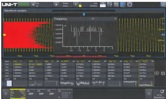
Standard enhanced FFT, up to 4 Mpts, 4 channels signal analysis
