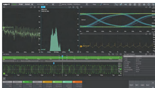
Jitter Analysis & Eye Diagram. Efficient measurement of clock and serial bus
