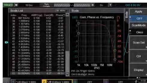
Provides a Bode plot for loop analysis
