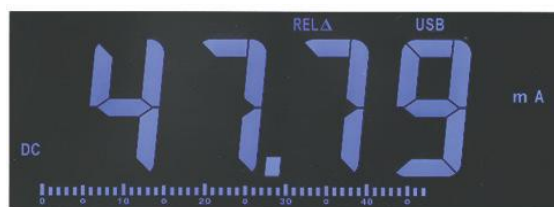
Extreme value operation and reference value operation function, with analog bar
