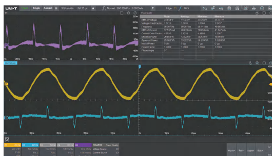
Power Measurement & Analysis. Provides a full range of analytical tools and assessment results
