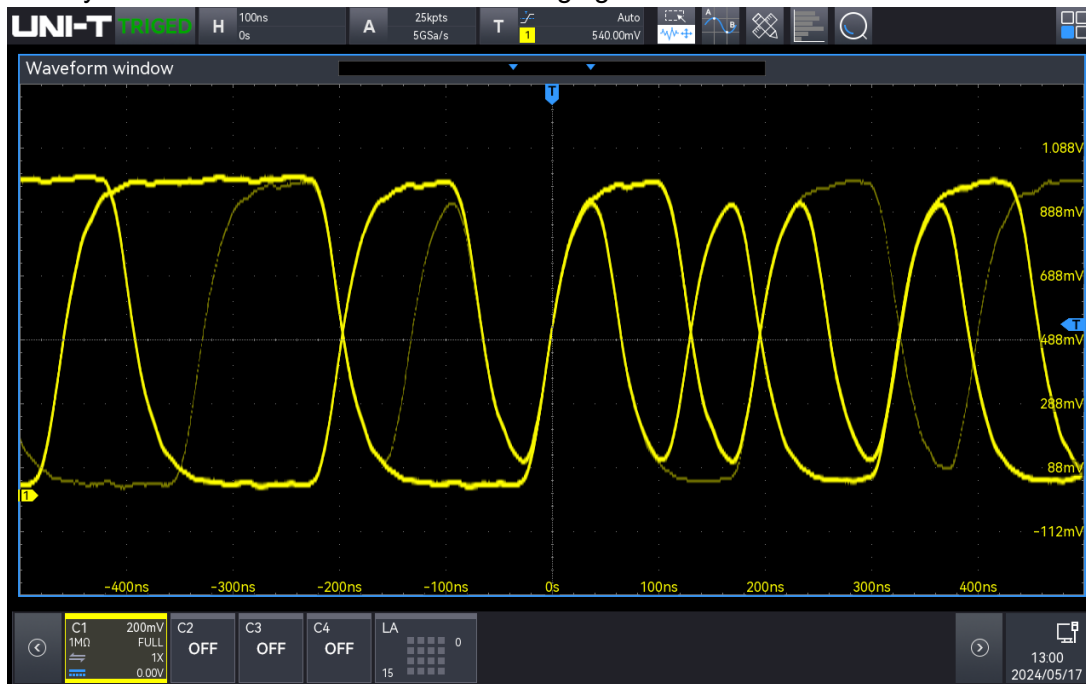
Serial data with jitter
