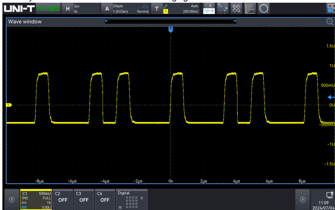
Repetitive pulse with ringing
