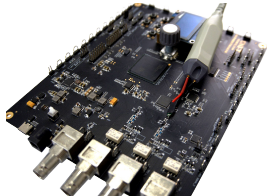
UT-PD2500 connects to MSO7000X and features a flexible front-end connector for connecting to the DUT.
