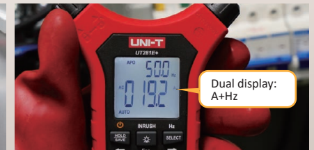
AC Current measurement
