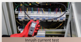
Inrush current test
