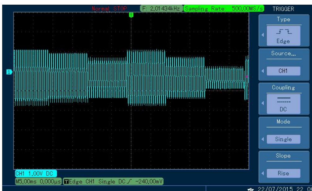
Figure 4- 98 Observe QAM waveform with oscilloscope
