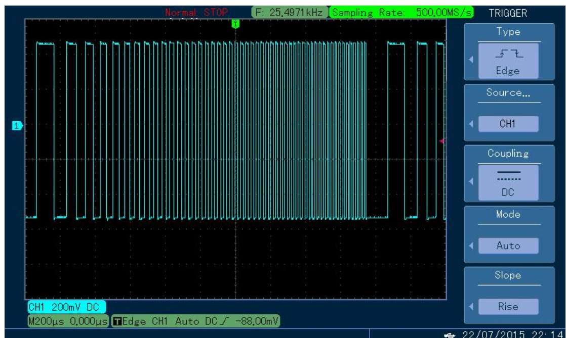
Figure 4- 132 Observe frequency sweep waveform with oscilloscope
