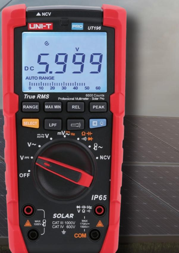
UT196 True RMS solar digital multimeter is an ideal tool for solar power system maintenance. This rugged meter is designed for technicians who work in rugged outdoor environments. UT196 can measure up to 1700V DC and 1500V AC voltages, and 3000A AC current with an external current clamp sensor. This solar meter offers IP65 protection and able to withstand 2m drop as well.
