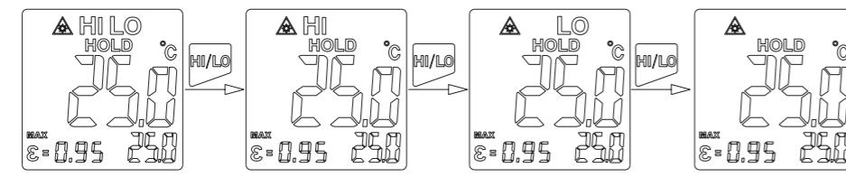
When the alarm function is on, alarm will go off when the temperature goes over the limit value. If measured temperature is higher than HI alarm limit, red LED and display will flash. If measured temperature is lower than LO alarm limit, blue LED and display will flash.
