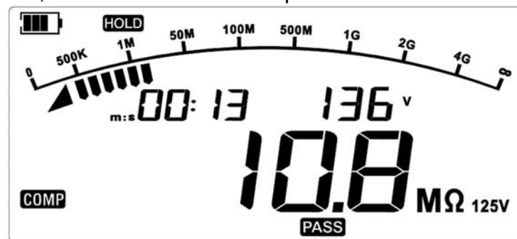
Figure 9.11 Comparative resistance measurement (10.0MΩ) is PASS
