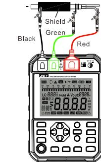
Fig. 10.1.3 Three-wire connection
