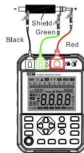
Fig. 10.1.2 Three-wire connection
