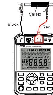
Fig. 10.1.1 Two-wire connection
