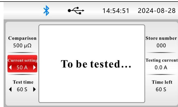
Figure 9.4 Output current setting
