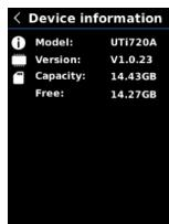
In the system settings interface, press the Up/Down button to select "Device information", and press the SET button to enter its submenu. The Model version/ Capacity/Free can be viewed. Press the Return button to return to the previous interface.
