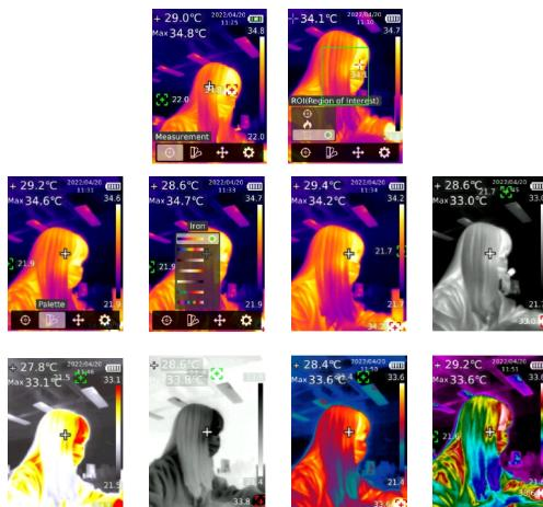
In the main interface, press the SET button to open the main menu. Press the Left/ Right button to select "Palette", and press the SET button to open its submenu. Press the Up/ Down button to select a palette. Press the SET button to use the selected palette. Press the Return button to return to the previous interface.
