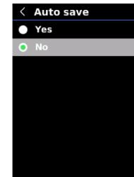
In the system settings interface, press the Up/Down button to select "Auto save", and press the SET button to enter its submenu. Press the Up/Down button to select Yes/No, and press the SET button to confirm. Press the Return button to return to the previous interface.
