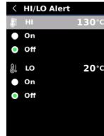
In the Settings interface, press the Up/Down button to select "HI/LO alert", and press the SET button to enter the alert setting interface. Press the Up/Down button to select On/Off. Press the SET button to set the alert value. Press the Up/Down button to add/subtract. Press the Return button to return to the previous interface.
