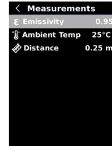
In the Settings interface, press the Up/Down button to select "Measurements", and press the SET button to enter its setting interface. Press the Up/Down button to select Emissivity /Ambient temp/Distance, and press the SET button to set the selected parameter. Press the Up/Down button to add/subtract the value, and press the SET button to confirm. Press the Return button to return to the previous interface.
