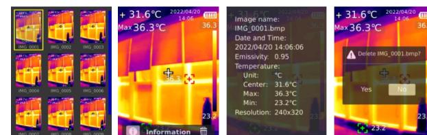
Press the Image Viewing button to view the images. Press the Up/Down/Left/Right to select an image, and press the SET button to view the image. Press the SET button again to view the image information and delete images.
