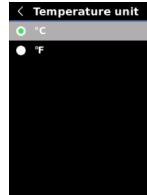
In the Settings interface, press the Up/Down button to select "Temperature unit", and press the SET button to enter the unit setting interface. Press the Up/Down button to select °C/°F, and press the SET button to confirm. Press the Return button to return to the previous interface.
