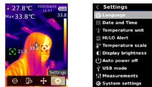
In the main interface, press the SET button to open the main menu. Press the Left/ Right button to select "Settings", and press the SET button to open its submenu. Press the Up/ Down button to select an option in the submenu, and press the SET button to enter its setting interface. Press the Return button to return to the previous interface.
