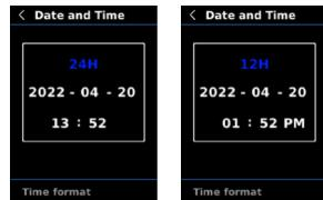
In the Settings interface, press the Up/Down button to select "Date and time", and press the SET button to enter its setting interface. Press the Left/Right button to select time format/year/month/day/hour/minute, and press the SET button to set the selected value. Press the Up/Down button to add/subtract, and press the SET button to save the modified value. Press the Return button to return to the previous interface.
