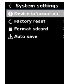
In the Settings interface, press the Up/Down button to select "System settings", and press the SET button to enter its setting interface. Press the Up/Down button to select Device information/Factory reset/Format SD card/Auto save, and press the SET button to enter the submenu. Press the Return button to return to the previous interface.
