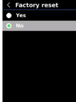
In the system settings interface, press the Up/Down button to select "Factory reset", and press the SET button to enter its submenu. Press the Up/Down button to select Yes/No, and press the SET button to confirm. Press the Return button to return to the previous interface.
