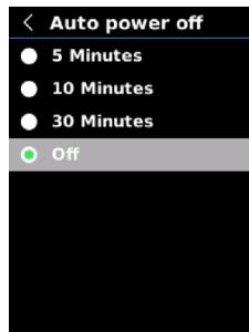
In the Settings interface, press the Up/Down button to select "Auto power off", and press the SET button to enter its setting interface. Press the Up/Down button to select 5 minutes /10 minutes/30 minutes/Off, and press the SET button to confirm. Press the Return button to return to the previous interface.
