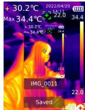
Press the trigger to capture an image. Press the Left/Right button to save it or not, and press the SET button to confirm or the Return button to cancel. In the auto save mode, the images will be automatically saved to the SD card.
