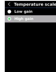
In the Settings interface, press the Up/Down button to select "Temperature scale", and press the SET button to enter the scale setting interface. Press the Up/Down button to select Low gain/High gain, and press the SET button to confirm. Press the Return button to return to the previous interface.
