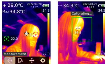
In the main interface, press the SET button to open the main menu. Press the Left/ Right button to select "Measurement", and press the SET button to open its submenu. Press the Up/Down button to select Center spot/Hi/Lo spot/ROI. Press the Return button to return to the previous interface.
