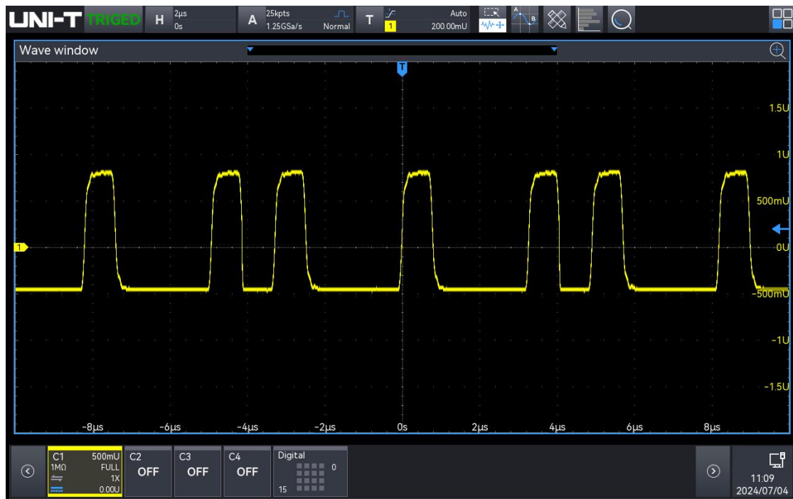
Repetitive pulse with ringing
