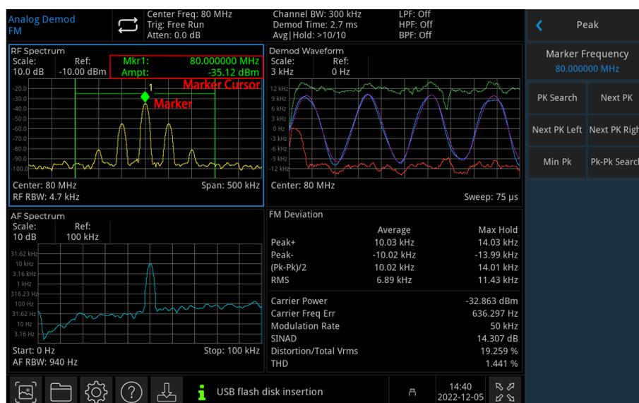
Figure 3-1 Reading of Marker Cursor Reading
