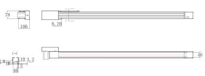
注:底部安裝位置可選裝在46的位置要求打M5固定牙孔. Note: the installation position at the bottom can be optional. M5 fixed tooth hole is required at the position of 46
