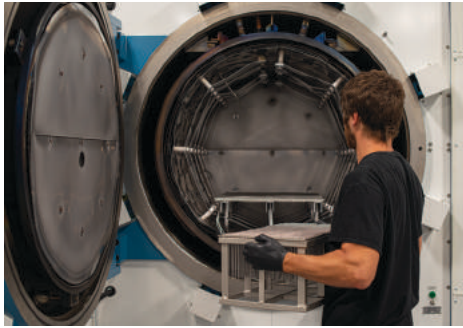
Vacuum Heat Treating
