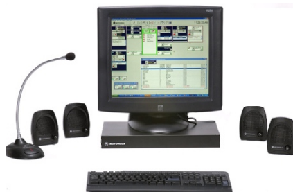
Figure 1-2: MCC 7500 Typical Operator Position
