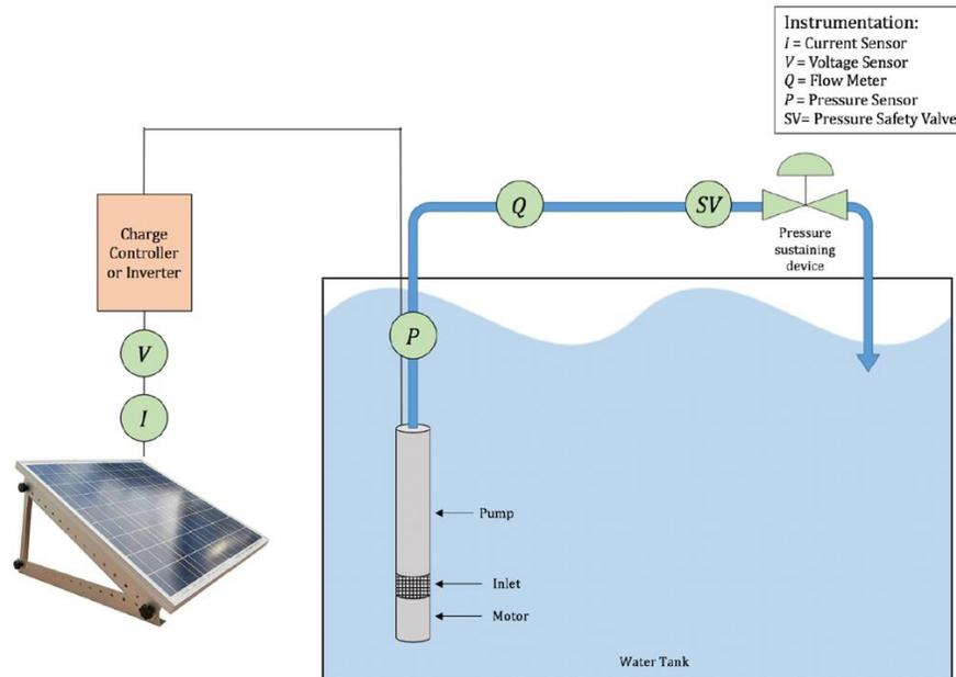
Figure 5: Alternative Test Set-Up
