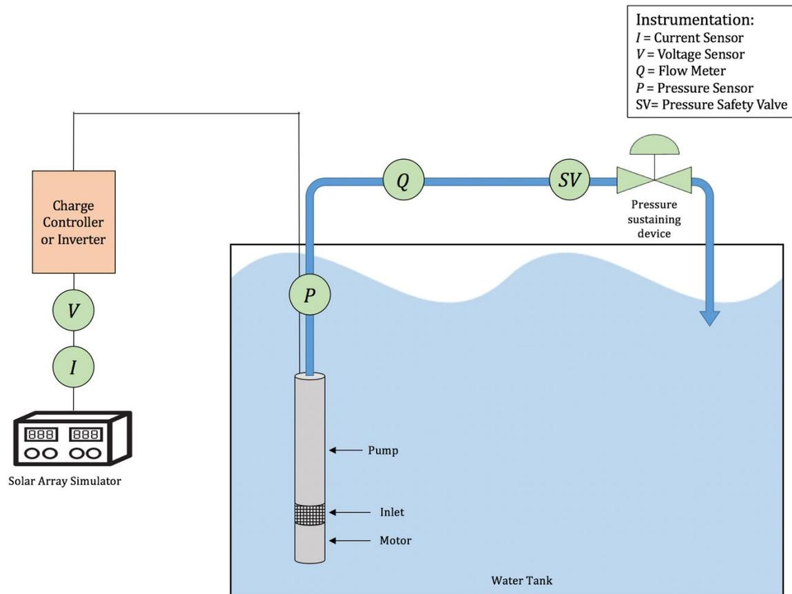
Figure 1: Test station diagram
