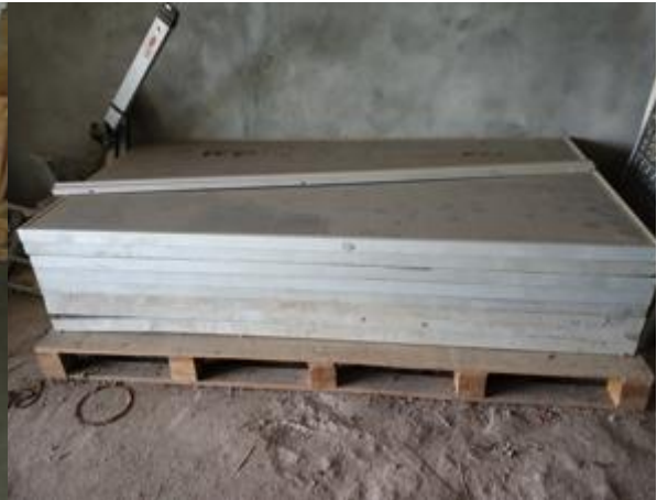
Incorrect storage of PV modules
