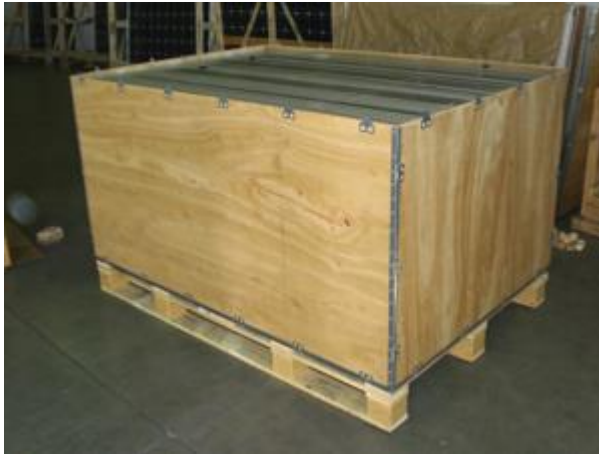
Correct storage of PV modules
