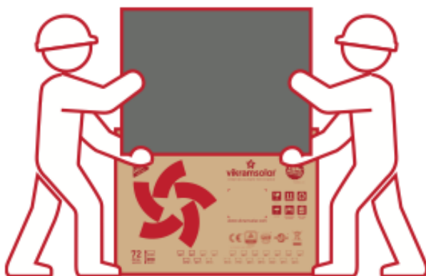
FIGURE 7: CORRECT WAY OF UNPACKING OF MODULES (SOURCE: VIKRAM SOLAR)
