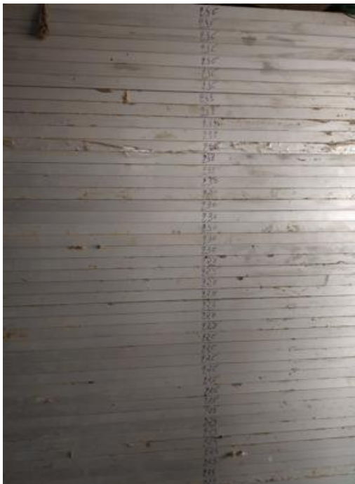
FIGURE 8: INCORRECT STORAGE OF MODULES - THIS MAY CAUSE IRREPARABLE DAMAGE TO THE MODULES
