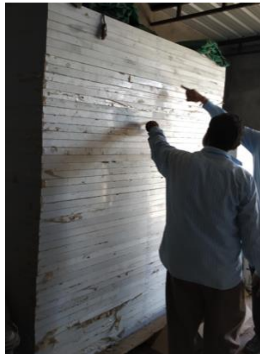
FIGURE 8: INCORRECT STORAGE OF MODULES - THIS MAY CAUSE IRREPARABLE DAMAGE TO THE MODULES
