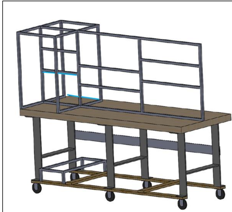
Figure 30. Blue indicating where the 23mm mounting track should be affixed to the t-slotted railing segment and butcher block utilizing t-nuts and hex screws, or washers and hex bolts, respectively.
