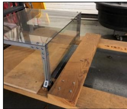
Figure 34. Polycarbonate shield box built to protect the Chroma from water exposure (note: Chroma not pictured here). To secure this "box", gussets, elbow supports, hex screws, and t-nuts are utilized along the t-slotted framing. The base of the framing is bolted to the wooden base
