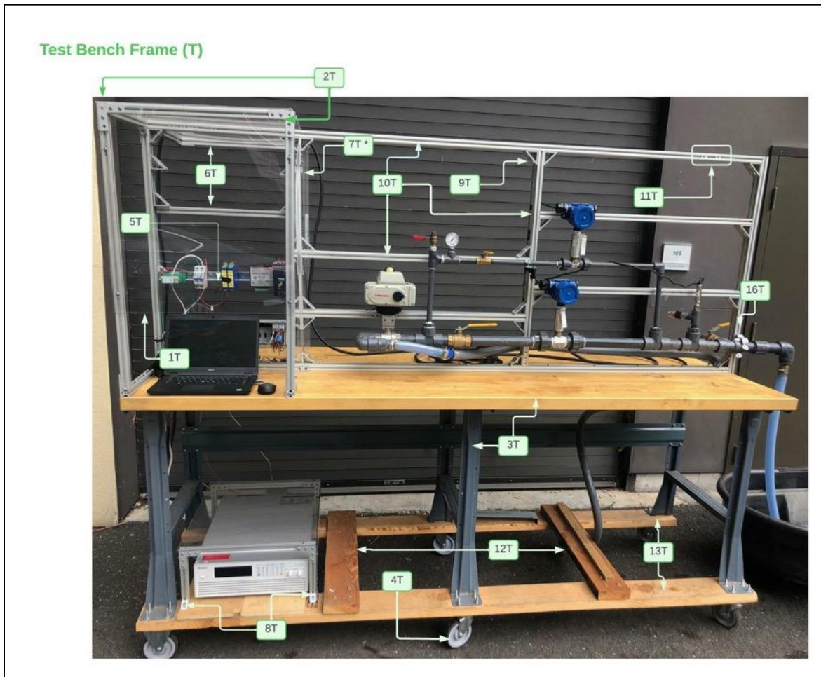
Figure 5. Test bench photo displayed with integrated equipment to frame.
