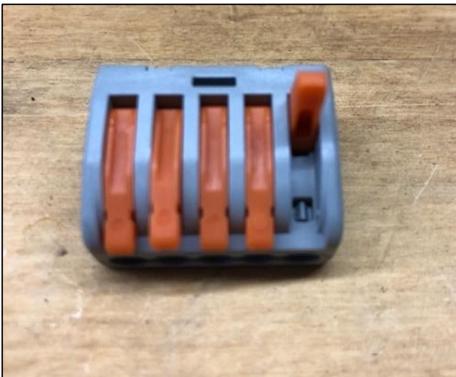
Figure 50. WAGO clamp connector- used throughout DAQ network as permanent connections, but also used in various non-permanent connection applications
