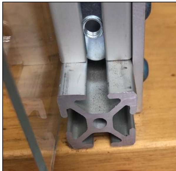
Figure 25. T-slotted framing base is bolted directly to the surface of the butcher block bench and t-nuts are slide into the framing grooves prior to connecting both ends of each segment in the test bench
