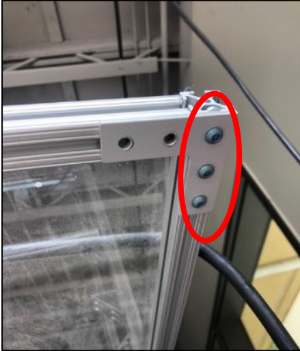
Figure 31. polycarbonate sheet affixed between t-slotted framing using hex screws, t-nuts, and elbow gusset
