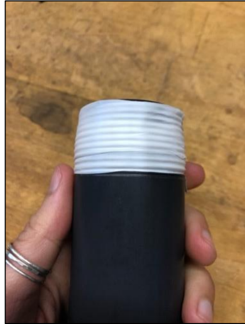
Figure 36. Layered and wrapped plumber's tape on male-end of a PVC adapter
