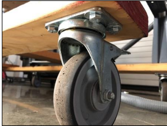
Figure 11. Wheels installed on casters that are bolted to the underside of the wooden base- there are six wheels total.
