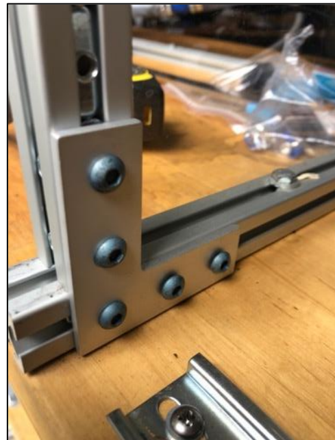
Figure 29. T-slotted framing held together in the bottom corner with 1 elbow support, and 5 hex screws, and 5 t-nuts. The base framing is bolted into the surface of the butcher block
