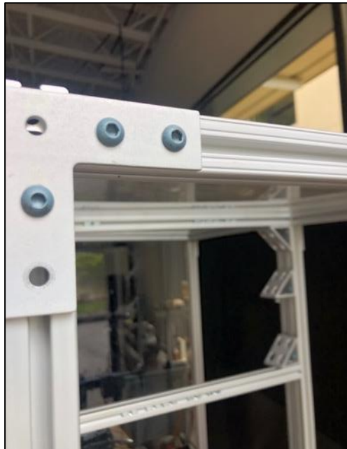
Figure 28. T-slotted framing held together in the corners with an elbow support, 3 hex screws, and 3 t-nuts- the screws are also going through a polycarbonate sheet here (more could be used here)
