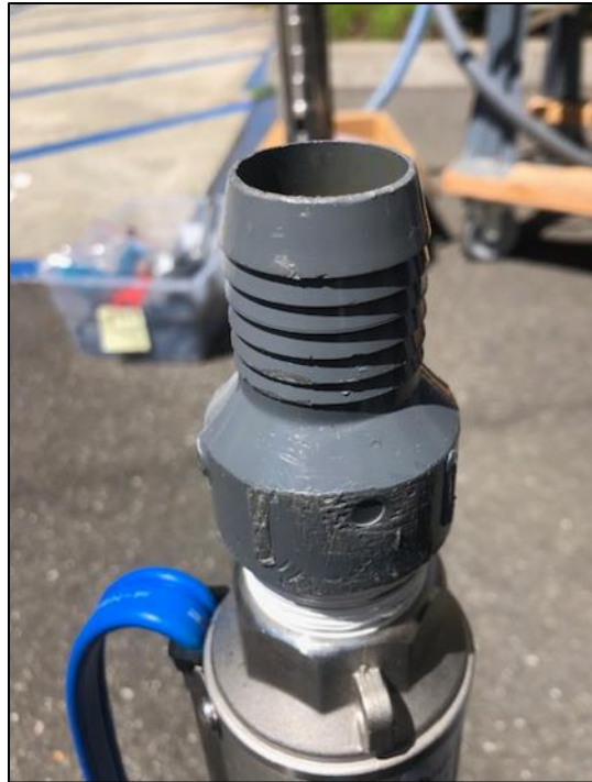
Figure 54. PVC adapter affixed to a SWP outlet so that it may be connected to the 3/4" threaded hosing inlet of the test bench piping network (notice the tub of various-sized PVC adapters sitting in the background that is kept on-hand for testing)
