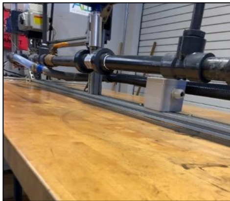
Figure 18. Base of the t-slotted framing bolted directly to the butcher block down the center of the surface to build the rest of the metal frame upon
