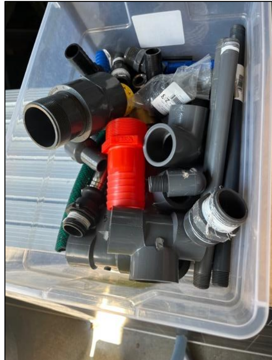
Figure 56. Adapters that can be used for connecting various sizes of pump outlets to the static diameter of the test bench inlet
