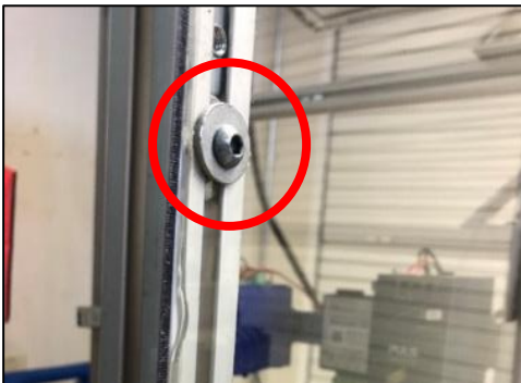
Figure 33. Polycarbonate shield installed on the t-slotted framing by drilling a hole and attaching with a hex screw twisted tight to a t-nut with a washer in-between the screw and the sheet
