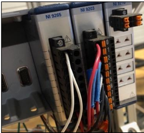
Figure 46. Clamp connections for wiring the NI DAQ
