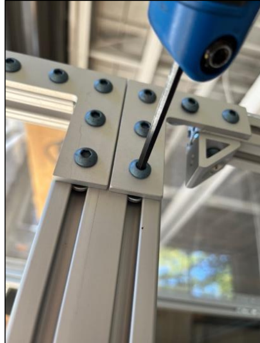
Figure 23. Some of the outer perimeter railing utilizes L-shaped gussets, which are affixed using an Allen wrench, hex screws, and t-nuts that are slid into the railing's slot.
