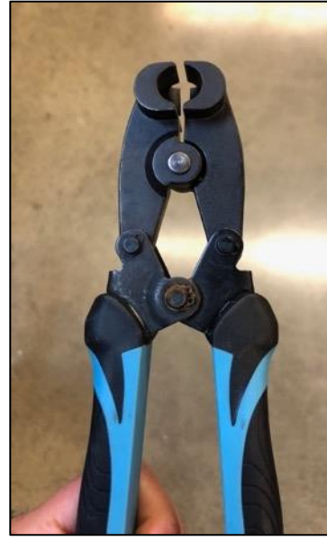
Figure 38. Pinch clamp pliers used for making permanent connections with ear hose clamps
