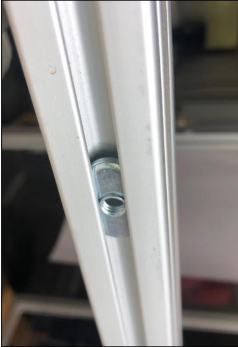
Figure 22. t-slot nut that is used to secure equipment onto the framing with a hex screw
