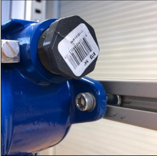
Figure 40. Flow meter attached to the t-slot framing via a t-slot nut and hex screw affixed through the racking hole on both sides of the meter
