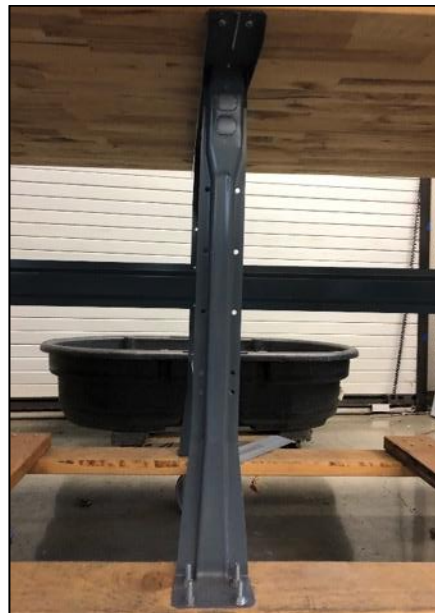
Figure 10. Metal legs bolted to the wooden frame directly over the wheels (underneath the wooden frame)
