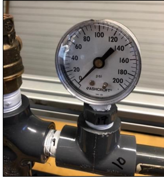
Figure 41. Pressure gauge connected in-line with PVC network. Because it is small and light in weight, it does not need to be secured to PVC network via t-slot nut and hex screw
