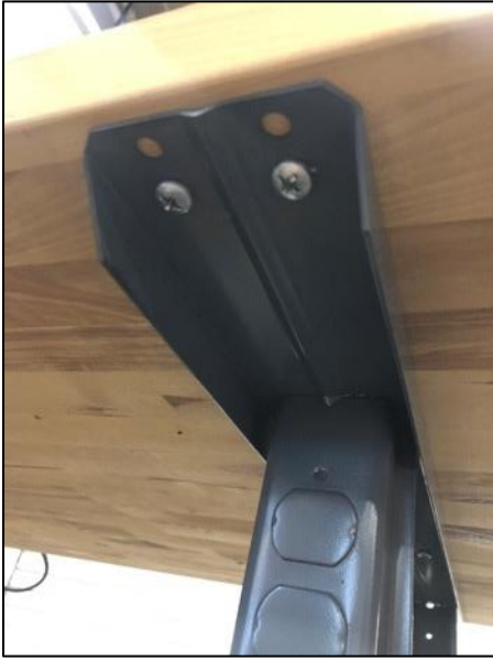
Figure 13. SWP test bench metal legs screwed to the underside of the butcher block table
