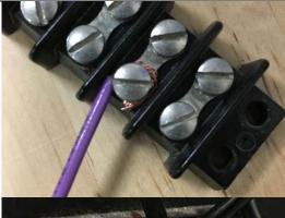
It is easy to fail to secure all the strands in this connection, which can increase the resistance of the connection or short with neighboring terminals.
