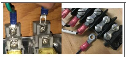
These connections are very secure but negate one of the advantages of using screw terminals, which is that the wire can be cut to size on-site.
