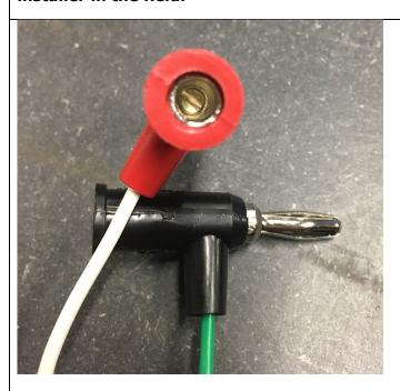
Only connectors with attachment mechanisms similar to those described above (wire is inserted into a hole and clamped down, binding posts, etc.) are considered acceptable. In the picture to the left, wire is inserted in the hole in the bottom of the plug and a set screw in the back of the plug is tightened to hold the wire in place.
