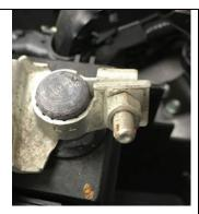
The wire must be either terminated at the factory or connected using one of the other acceptable methods listed in this document (such as clamped between two plates).
