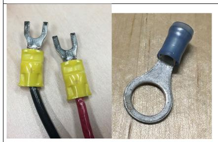
These connections can be more secure than those made with bare wire, but the installer must be trained in proper crimping technique and the tool, terminal, and wire size must all be matched, or a poor connection will result. In addition, training is needed to distinguish a good crimp from a poor crimp.
