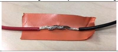
This is not an effective method for making reliable wire connections.
